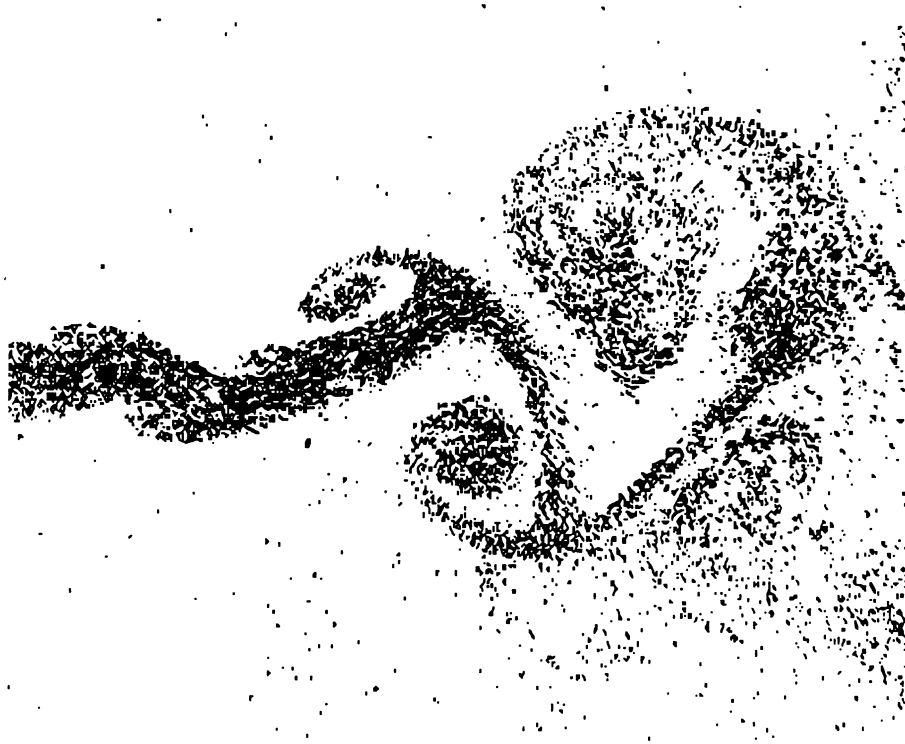
Fig. 2. A computer-enhanced image of tracer particles in a plane perpendicular to the jet slot for 4.8D \times 6.6D downstream from the jet exit at Re = 173 .
